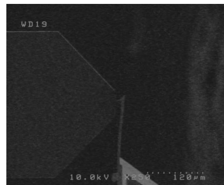
Fig. 1 – Deflecting an AFM cantilever with an FS-2000 force sensor mounted on a NanoBot
